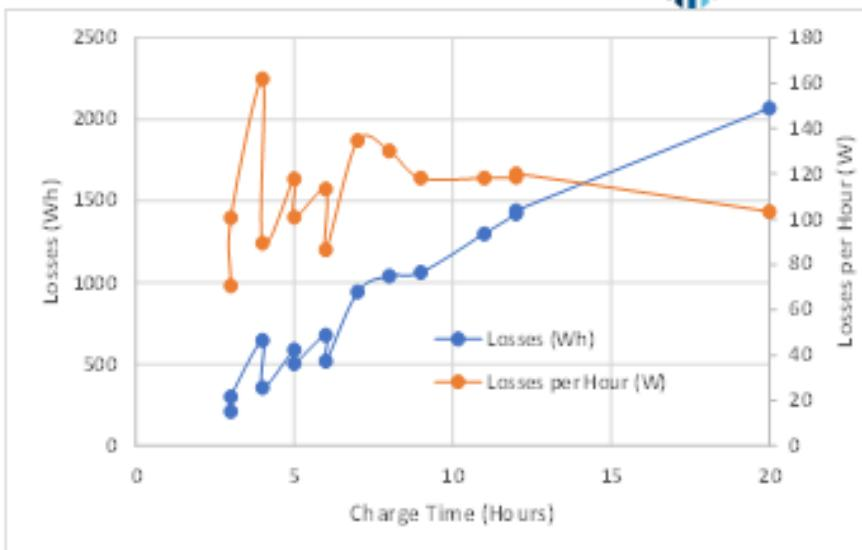
The Figure shows that the charging losses are directly proportional to the charge time. However, irrelevant to the charge time the losses per hour are averaging approximately at 113W.
