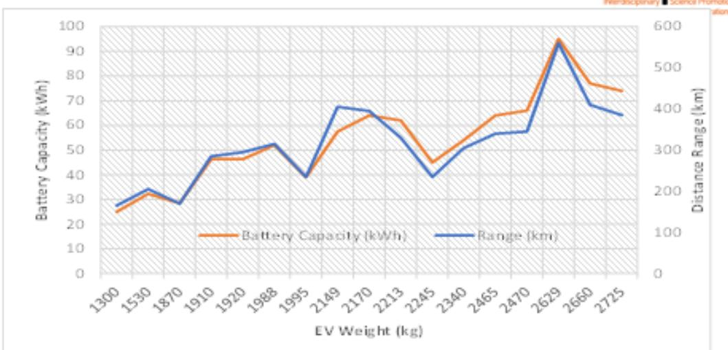
As the EV becomes bigger, then theoretically the payload increases which allows for bigger battery which leads to further driving distances.
